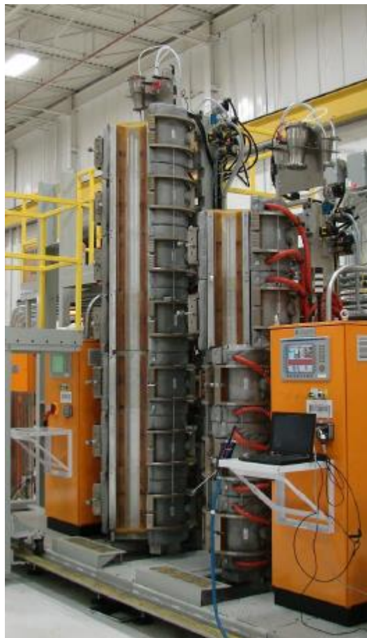
Figure 2: Vacuum Encapsulation - Resin Impregnation and Curing [6]
