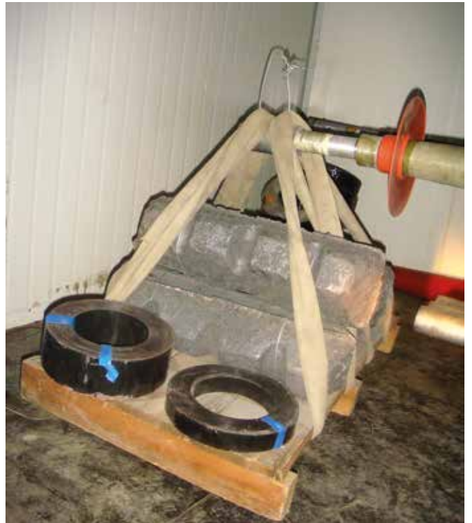
Figure 5. Cantilever load test at low temperature
