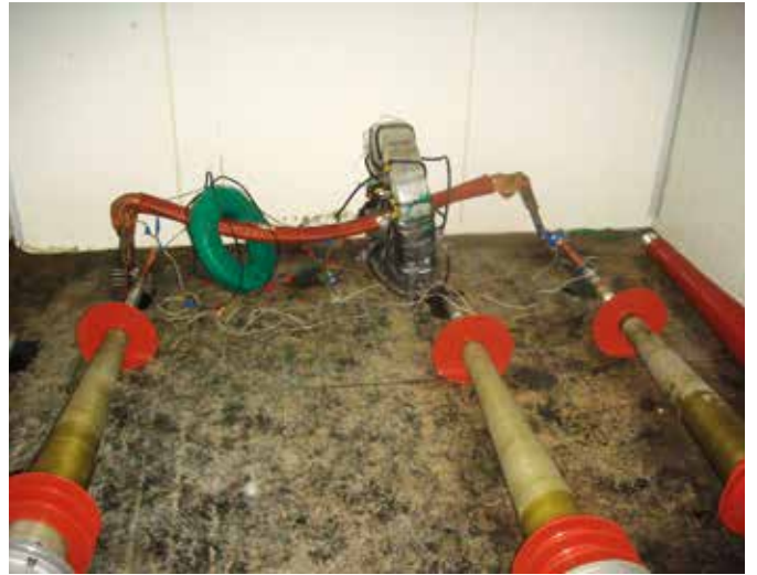
Figure 3. Low temperature test with current injection
