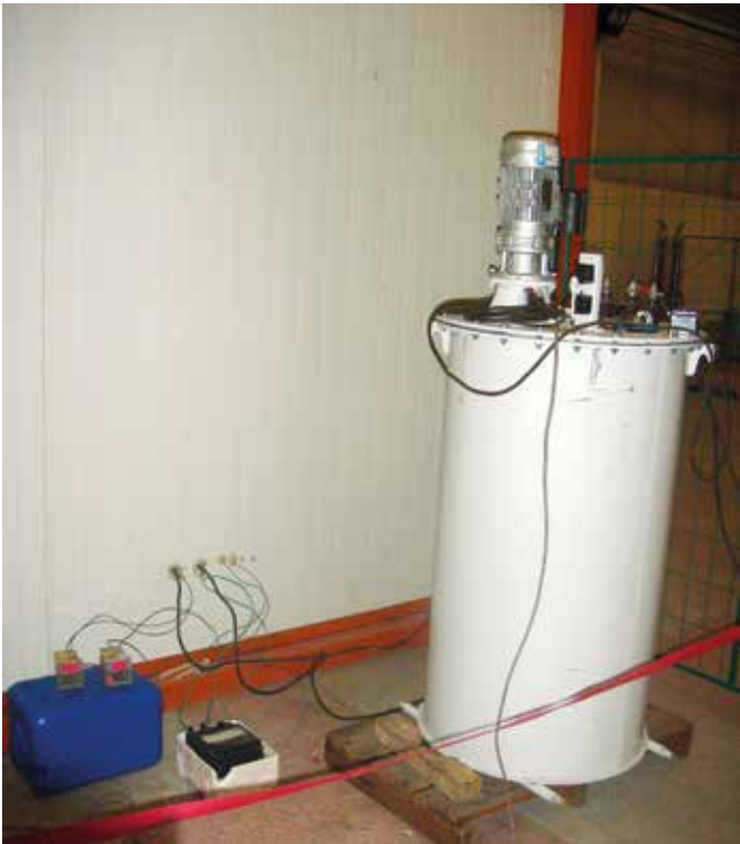
Figure 4. Low temperature test with current injection
