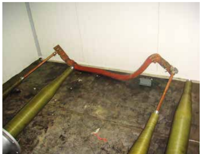
Figure 7. Low temperature test with current injected
