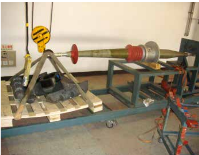
Figure 6. Heavy cantilever load test at 105 °C
