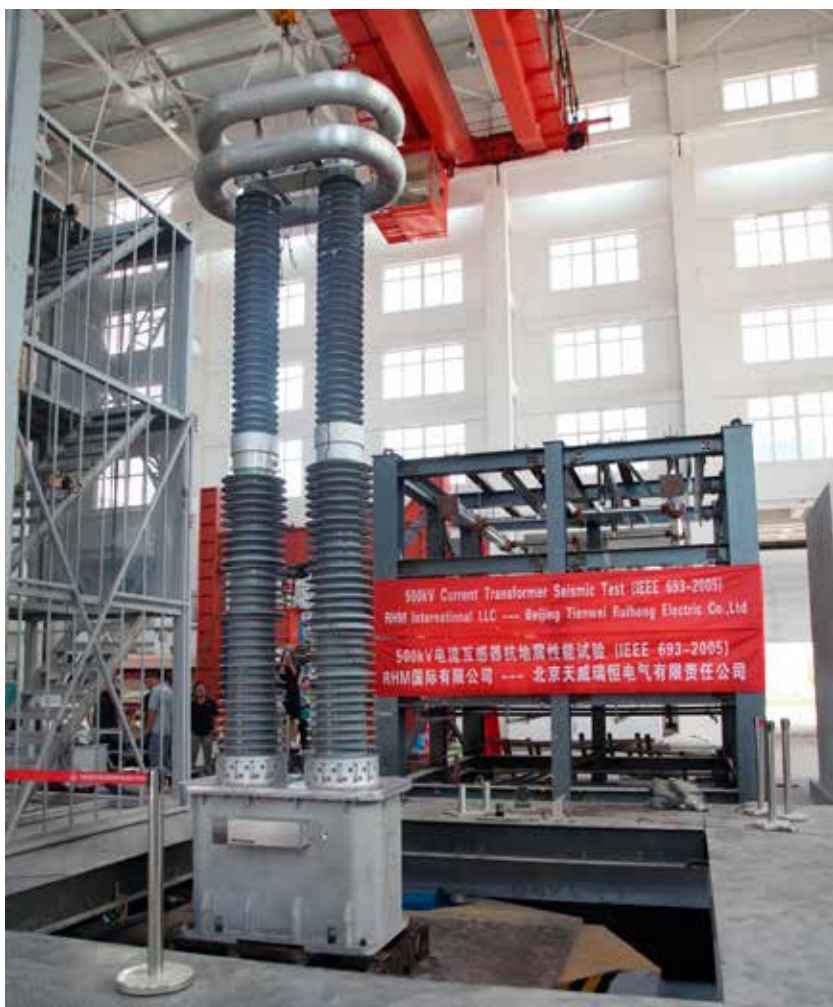
Figure 3 – 500 kV Dry type current transformer on shake table
