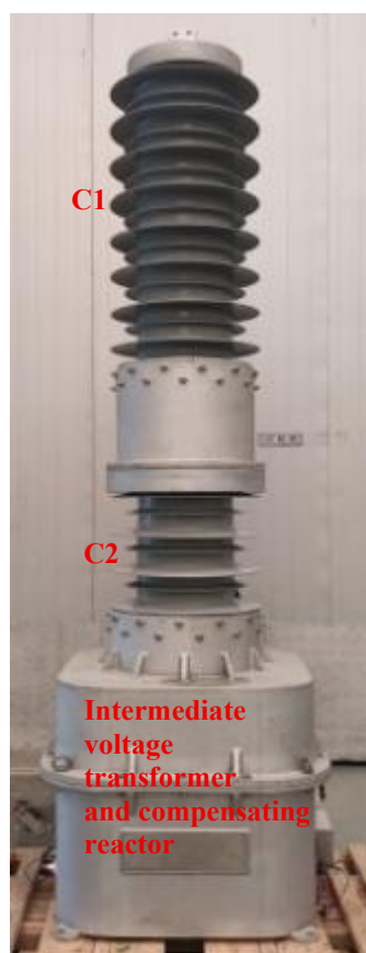
Figure 1 - 110kV GCVT prototype
